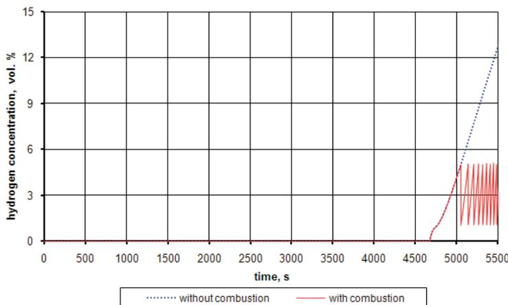
Figure 6. Hydrogen concentration within the leakage zone.
