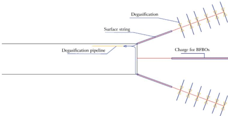
Fig. 7. Diagram of combined prevention method utilizing degasification and BFBOs – 2<sup>nd</sup> variant
