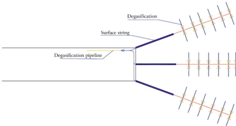
Fig. 3. Diagram of degasification method of prevention
