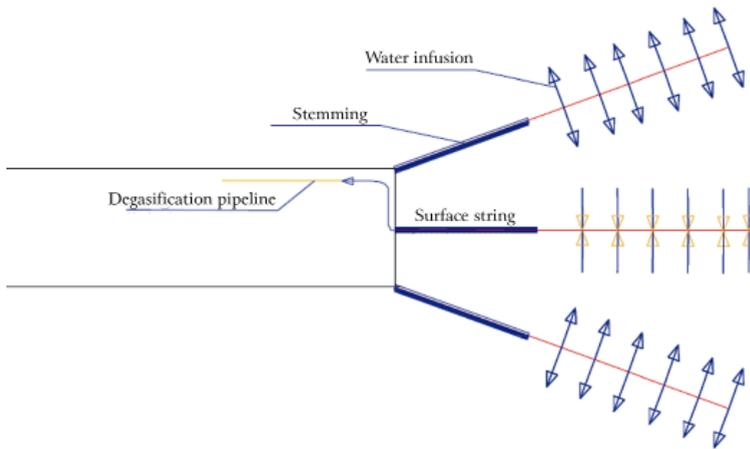
Fig. 4. Diagram of combined prevention method utilizing degasification and water infusion – 1<sup>st</sup> variant
