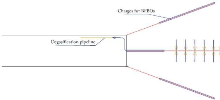
Fig. 6. Diagram of combined prevention method utilizing degasification and BFBOs – 1<sup>st</sup> variant
