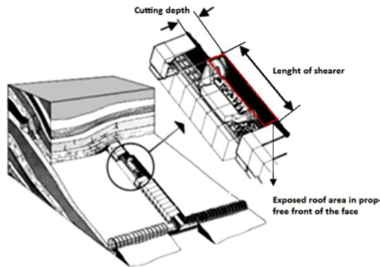
Fig. 1. Exposed roof area in prop-free front of the face in longwall mining (Saedi et al., 2010)
