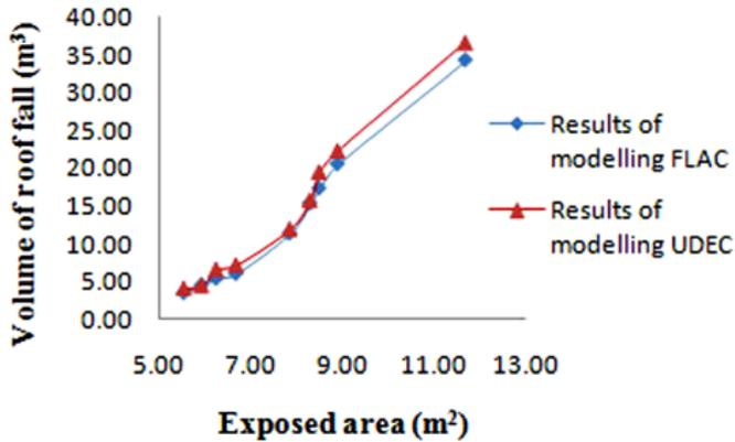
Fig. 8. The effect of exposed roof area on the volume of roof fall
