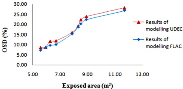
Fig. 9. The effect of exposed roof area on OSD
