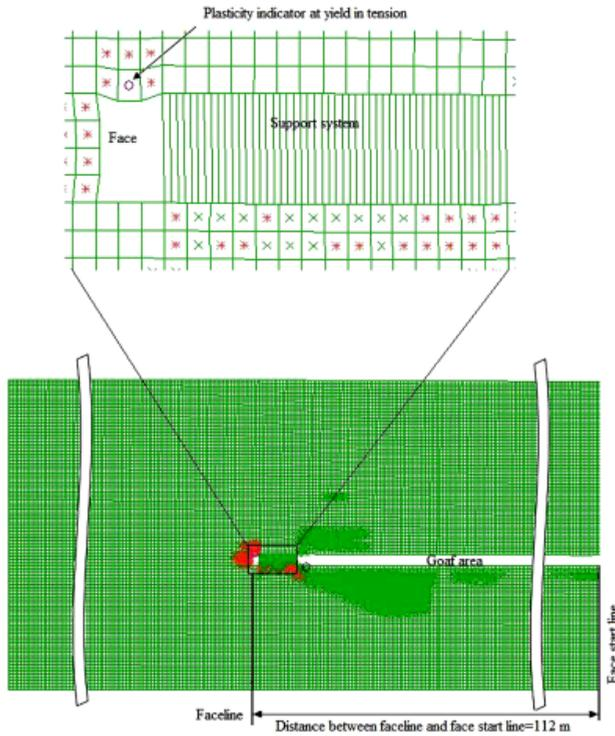
Fig. 4. Plasticity state indicator under yield tension for determination of OSD using FLAC<sup>2D</sup>
