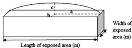
Fig. 2. Illustration of roof fall envelope in prop-free front of the face
