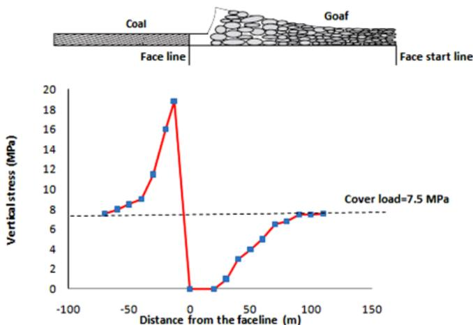
Fig. 6. A predicted model of vertical stress redistribution around a coal longwall face<sup>10</sup>
