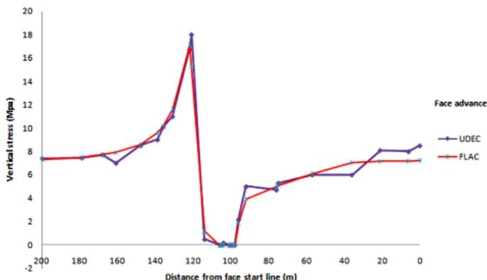
Fig. 7. Vertical stress distributions obtained from the model around the face and gob forming by using UDEC and FLAC
