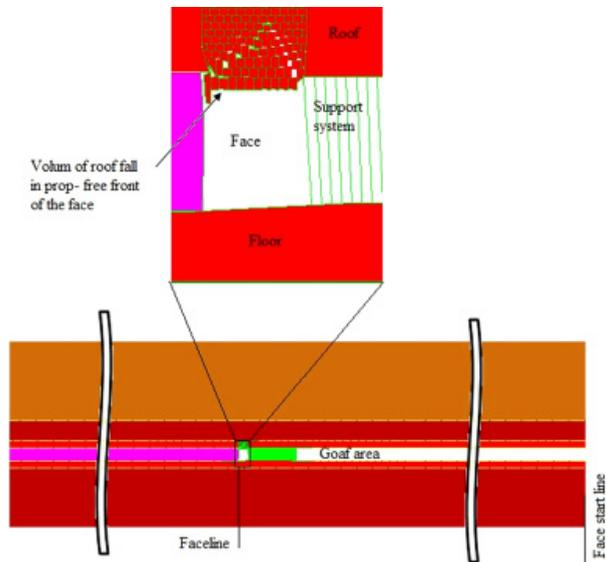
Fig. 5. Roof fall in front of the face for determination OSD using UDEC
