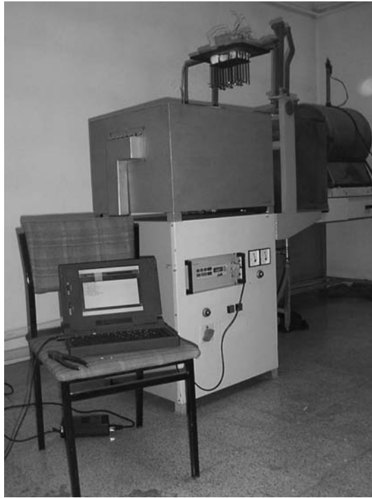
Fig. 7. The device for thermal fatigue testing of metals
