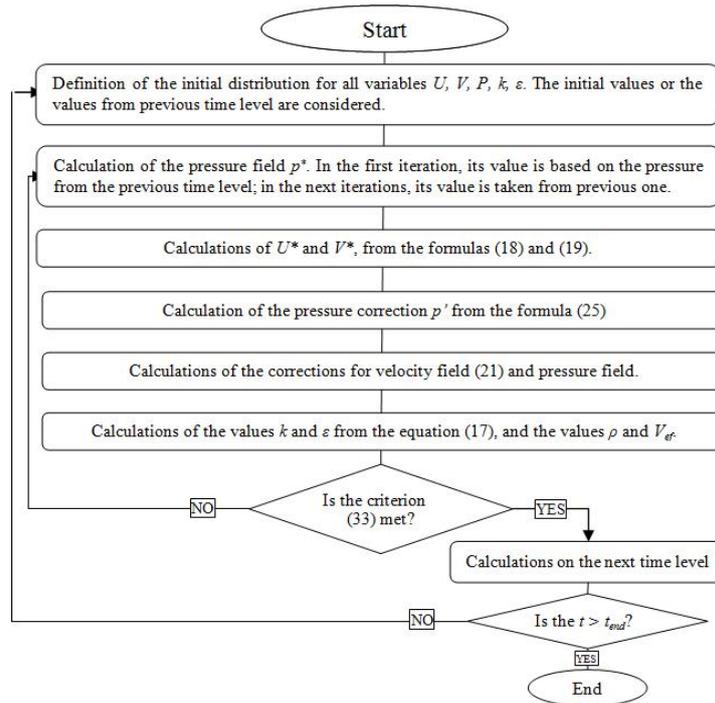
Fig. 5. The iteration algorithm.
