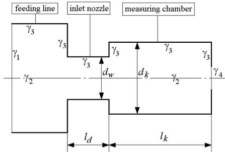
Fig. 3. The computational domain inside the air gauge measuring chamber.
