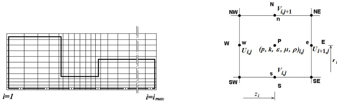
Fig. 4. Discretization of the calculation area.
