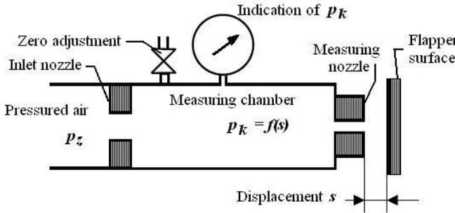
Fig. 1. Scheme of the typical back-pressure air gauge [3].
