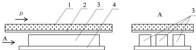
Fig. 3. Schematic of the experiment on copper plate drive on the steel samples with different hardness: 1 – explosive charge, 2 – copper plate, 3 – steel samples, 4 – base plate,  $D$  – detonation velocity
