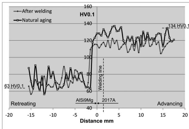
Fig. 7. Hardness distribution on the cross section of the weld – 3 mm from face of the weld; dashed line indicates the welding line (FSW tool position relative to the edge of the welded elements)
