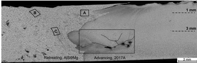
Fig. 2. Macrostructure of cross-section of the weld
