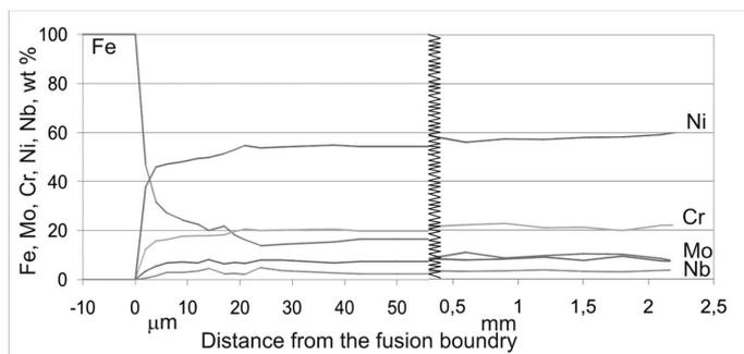
Fig. 3. Distribution of Fe, Ni, Cr, Mo, Nb (wt %) as a function of the distance from the fusion boundary
