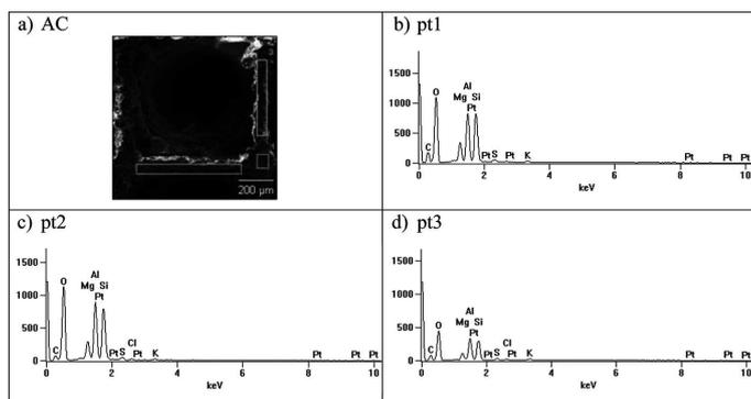
Fig. 2. SEM microphotograph of AC surface (a) and microanalysis of chemical composition in marked areas: pt1 – pt3 (b-d)
