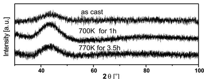
Fig. 1. The X-ray diffraction patterns of the investigated  $Fe_{61}Co_{10}Y_8Ni_1B_{20}$  alloy in the as-quenched state and after isothermal annealing
