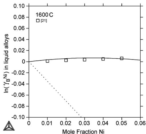
Fig. 9. Calculated activity coefficient  $\gamma_B^{Ni}$  in liquid Fe-B-Ni alloys at 1600°C, together with smoothed experimental data points [21]. Solid lines refer to the current calculations and dotted lines show those of [2]
