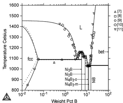
Fig. 3. B-Ni phase diagram calculated with the parameters obtained in this work, together with experimental data points [7-11]. Solid lines refer to the current calculations and dotted lines refer to those of Campbell and Kattner [4]
