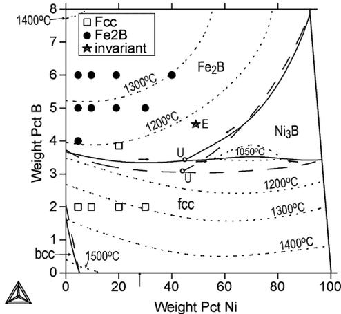
Fig. 4. Calculated liquidus projection of the Fe-B-Ni system, together with experimental data points [17, 5]. Solid lines refer to the current calculations and broken lines show those of [2]. Shown also are the calculated liquidus isotherms between 1050 and 1500°C, by dotted lines
