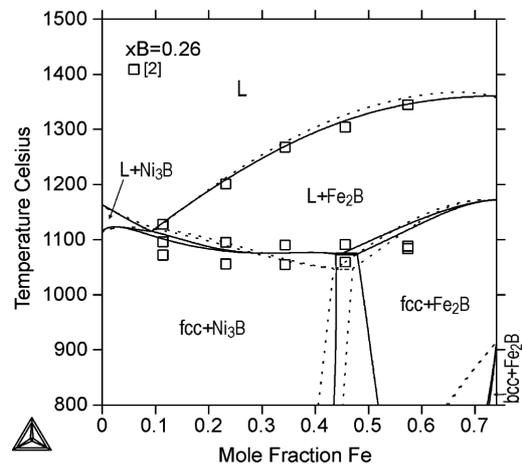
Fig. 7. Calculated vertical section at  $x_B = 0.26$  in the Fe-B-Ni system, together with experimental data points [2]. Solid lines refer to the current calculations and dotted lines show those of [2].  $x_B$  is the molar fraction of boron
