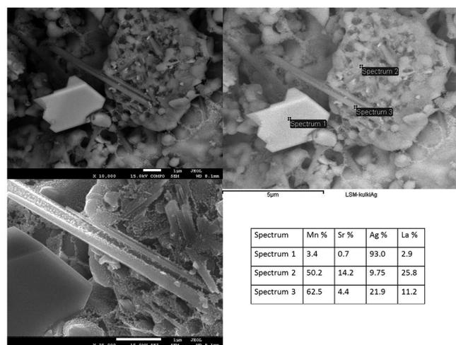
Fig. 2. SEM pictures at two different magnifications of the LSM cathode after introduction of silver and sintering, view from the top (left), and the picture in the reflected electron mode of the same area (right). In that mode the brightness of the picture is proportional to the atomic number of the element and the density of the material. Results of the EDS analysis performed at the particular points are also given in the picture in the form of a table
