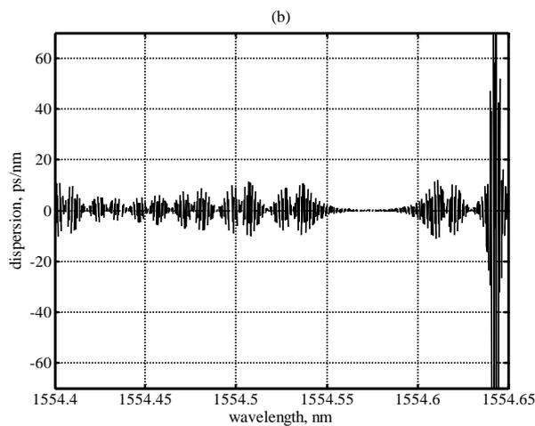
Figure 12. Characteristics obtained in the case of heterogeneous elongation of the compensator's grating. The maximum value of the grating's deformation =  $1.95 \cdot 10^{-5} \epsilon$ . The grating is apodized according to the Gaussian function ( $a=5$ ),
