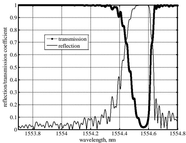
Figure 11. Transmission and reflection spectrum in the case of heterogeneous elongation of the compensator's grating. The maximum value of the grating's deformation =  $1.95 \cdot 10^{-5} \epsilon$ . The grating is apodized according to the Gaussian function ( $a=5$ )
