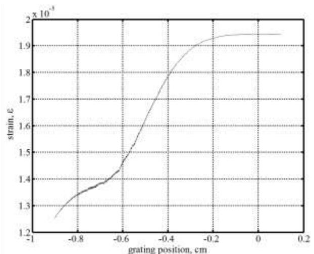
Figure 5. Distribution of deformation values along the grating. 0.9 – beginning of grating, +0.1 – end of grating
