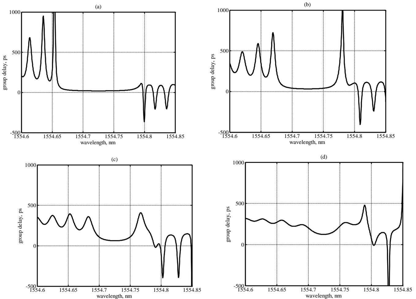
Figure 15. Graphs of group delay in the vicinity of the dispersion compensator's Bragg wavelength, (a) no apodization, (b) Gauss apodization,  $a=2$ , (c) Gauss apodization,  $a=5$ , (d) Gauss apodization,  $a=10$ .
