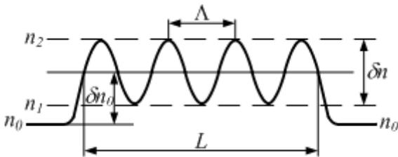
Figure 1. Designation of the characteristic parameters of the modulation of refractive index in the model dispersion compensator
