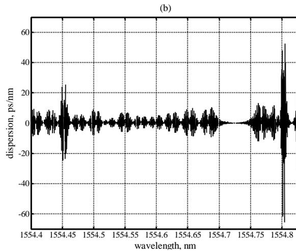
Figure 14. Reflection spectrum in the case of heterogeneous elongation of the compensator's grating. The maximum value of the grating's deformation =  $2.92 \cdot 10^{-5} \epsilon$ . The grating is apodized according to the Gaussian function ( $a=5$ ), (a) group delay, (b) dispersion
