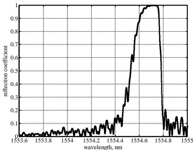
Figure 13. Reflection spectrum in the case of heterogeneous elongation of the compensator's grating. The maximum value of the grating's deformation =  $2.92 \cdot 10^{-5} \epsilon$ . The grating is apodized according to the Gaussian function ( $a=5$ )
