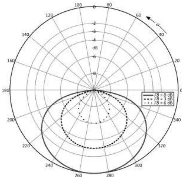
Fig. 6. The impact of  $FB$  variable on the main back lobe ( $HPBW_{back} = \text{constant}$ )
