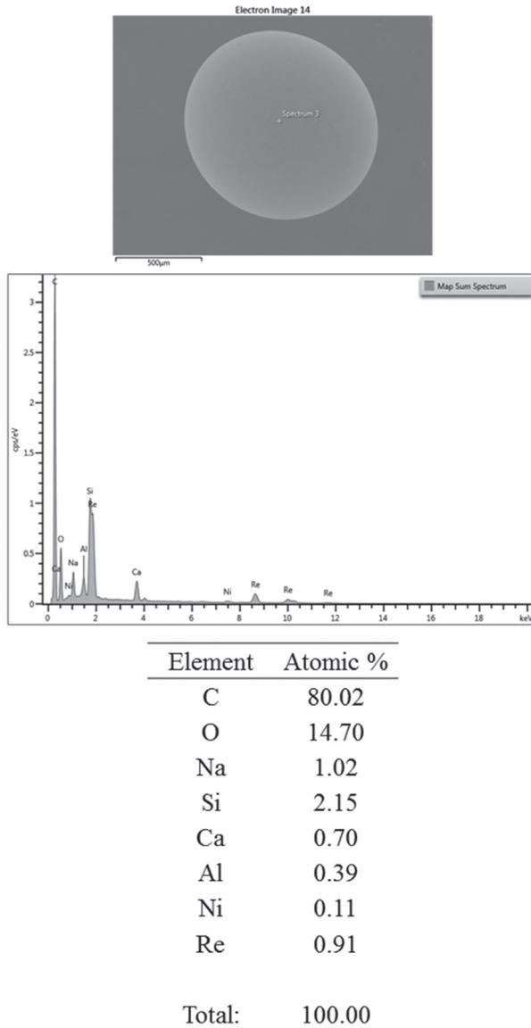
Fig. 2. Bead coated with rhenium nanolayer (top panel) and chemical composition of the bead surface revealed by the energy dispersive spectroscopy (EDS) method (bottom panels).
