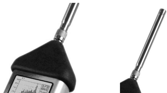
Fig. 2. Top of an SLM and a microphone placed on an extension.
