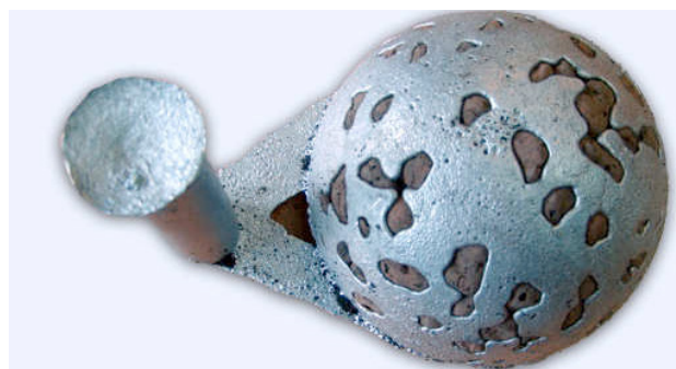
Fig. 5. Open pore casting before annealing VSB-TU Ostrava [5]
