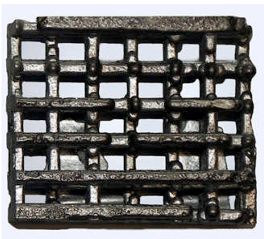
Fig. 3. Application of two stage investment casting for production of casting with regular cellular structure (obtained porosity 60-68%) at the Department of metallurgy and foundry VSB-TU Ostrava [5]
