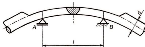
Fig. 1. The deformation of wires after longitudinal grinding to the half diameter [8]
