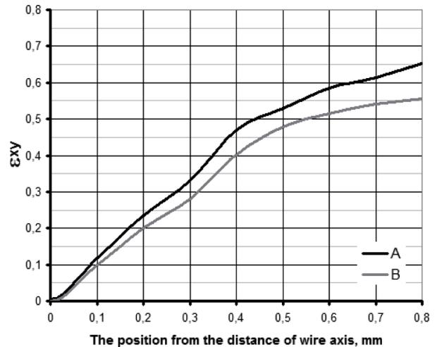
Fig. 9. The distributions of the redundant strain  $\varepsilon_{xy}$  on the cross-section of  $\phi 1.6$  mm wires drawn according to Variants A and B
