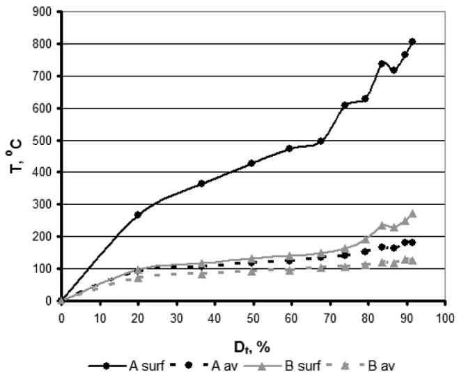
Fig. 6. The change of temperature on the surface and the axis after exit from the bearing zone of die for wires drawn according to variant A and B in total draft function
