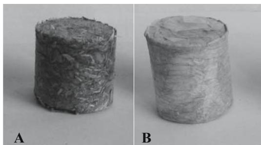
Fig. 1. Fuel based on oat straw with polyethylene: A – shredded, B – plain (photograph by M. Kajda-Szcześniak)
