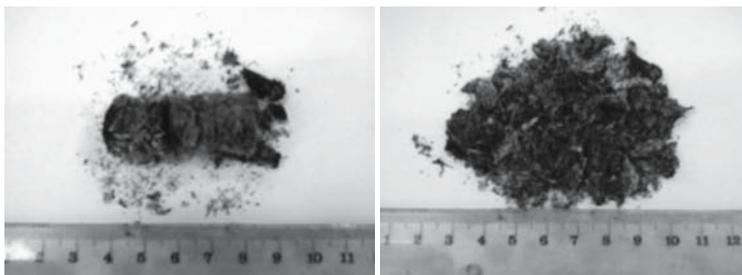
Fig. 4. Ash from burning fuel based on oat straw with the admixture of not shredded polyethylene (by M. Czop)
