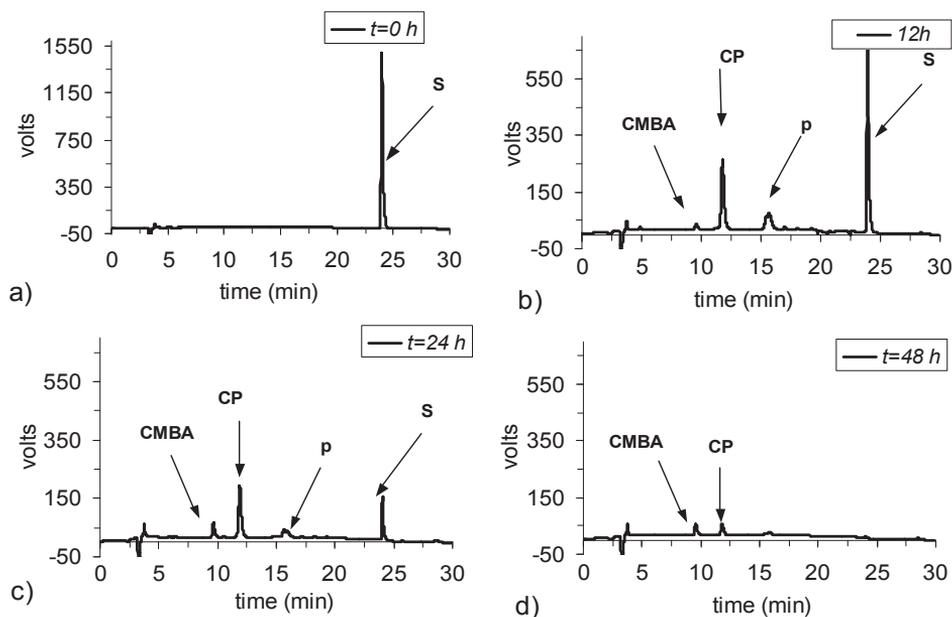
Figure 3. HPLC chromatogram (at 240 nm) of an irradiated aqueous solution of sulcotrione (pH 6.5). Sulcotrione conversion percentage: 0% (a), 47% (b), 90 % (c) and 100 % (d)
