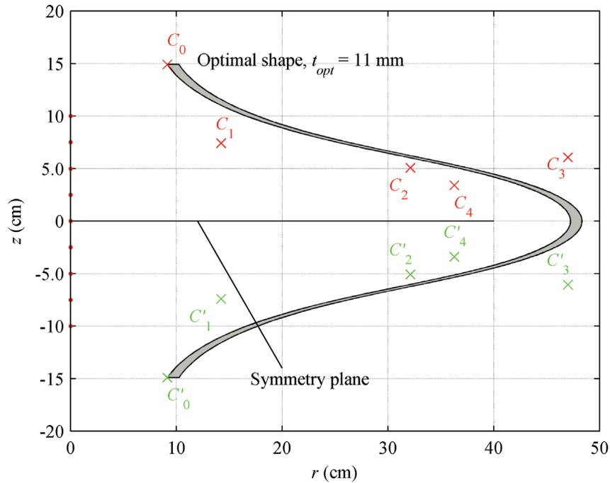
Fig. 6. Optimal shape of the solenoid for desired magnetic field  $H_0 = 45$  kA/m with determined  $t_{opt} = 11$  mm
