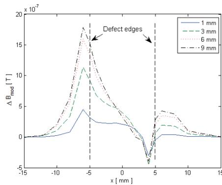
Fig. 4. Numerical simulation results: differential response signals using probe tilting in x-axis,  $\varphi = 45^\circ$  tilt
