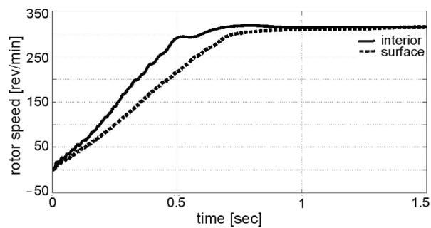
Fig. 7. Transient speed at no load
