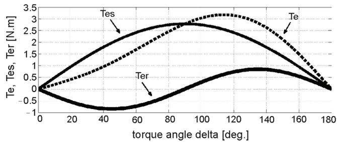
Fig. 15. Steady state torque components of IPMSM
