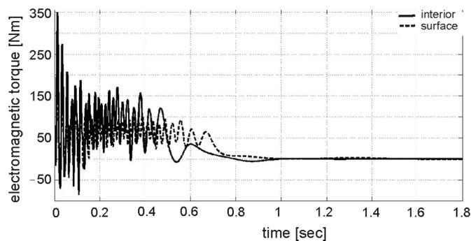
Fig. 9. Airgap torque dynamics at no load
