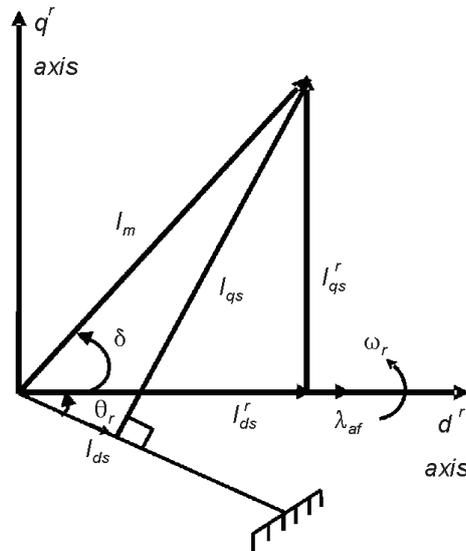
Fig. 6. Stator input current phasor diagram
