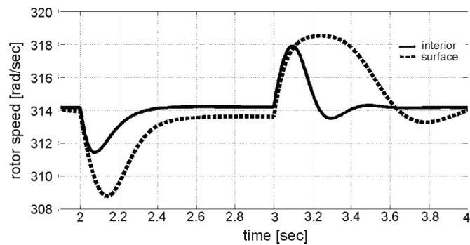
Fig. 8. Speed dynamics due to sudden load changes
