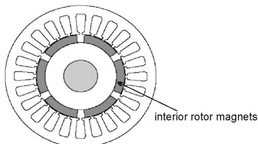
Fig. 2. IPMSM rotor assembly
