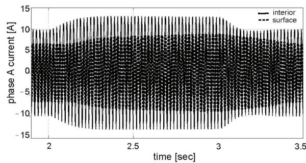
Fig. 12. Stator Current dynamics due to sudden load changes
