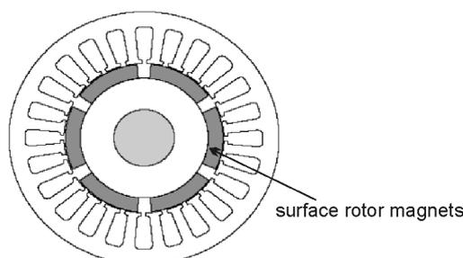
Fig. 1. SPMSM rotor assembly
