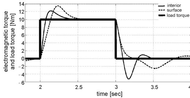
Fig. 10. Torque dynamics due to sudden load changes
