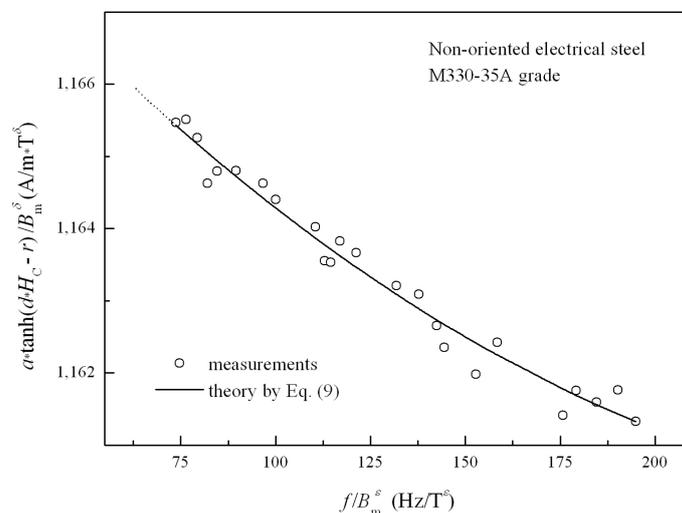
Fig. 3. Distribution structure of scaled data points for higher frequencies
