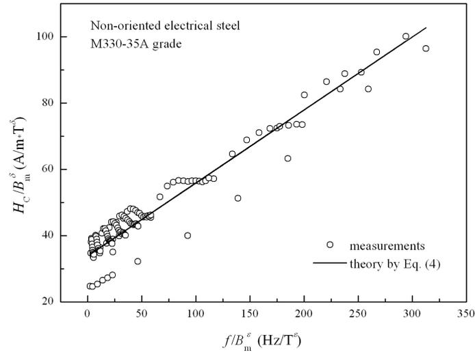
Fig. 1. The Widom-based scaling transformation of coercivity measurements for non-oriented electrical steel
