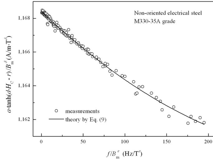
Fig. 2. The modified scaling transformation of coercivity measurements for non-oriented electrical steel
