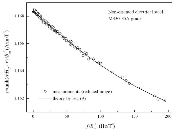
Fig. 4. The modified scaling transformation of coercivity measurements for non-oriented electrical steel in the case of reduced measurement data
