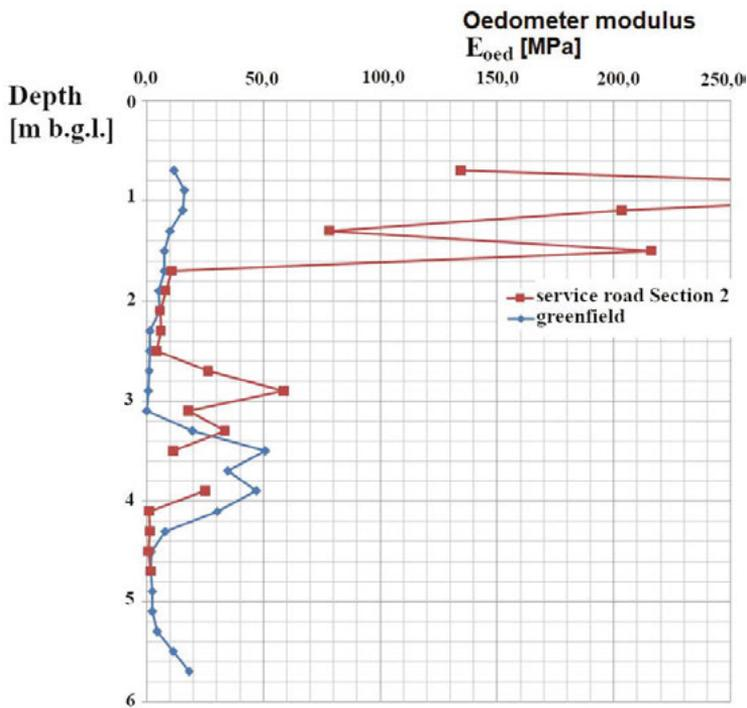
Fig. 6. Compressibility modules from the DMT tests in the substrate of section 2 and greenfield
