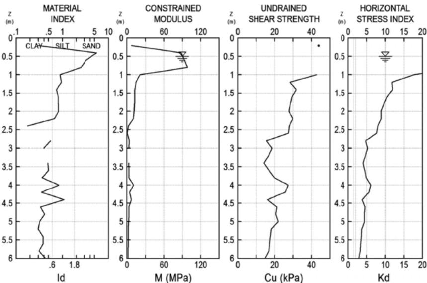
Fig. 4. DMT5 dilatometer test results [9]
