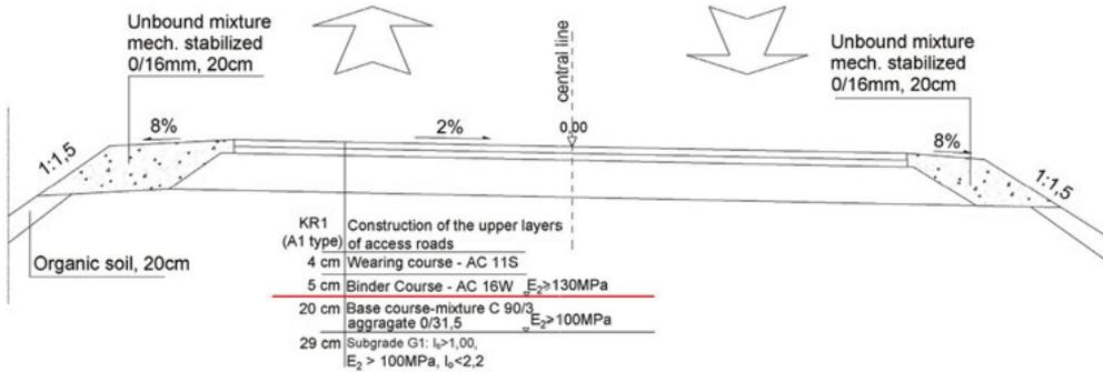
Fig. 1. Typical design section of the analyzed roads
