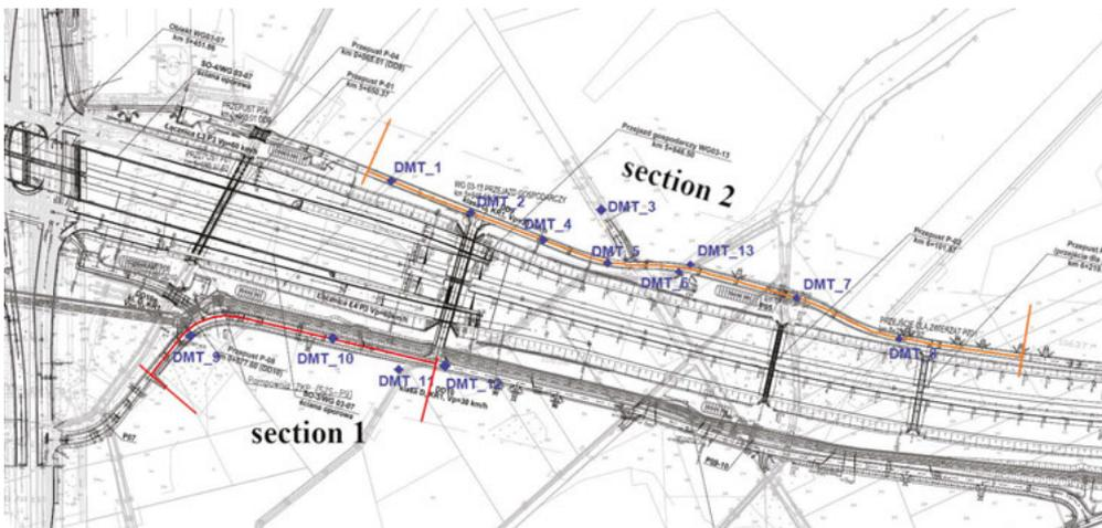
Fig. 2. The field tests DMT location map
