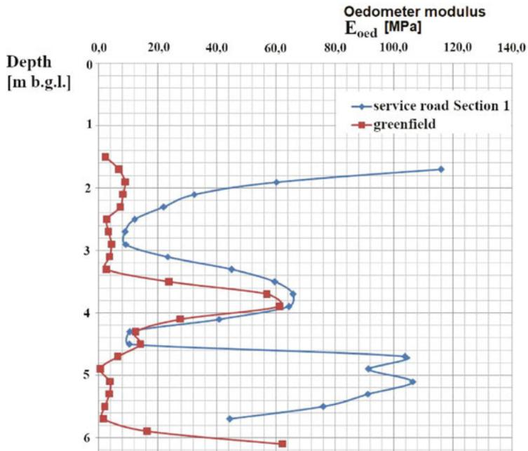
Fig. 5. Compressibility modulus from the DMT tests in the basement of section 1 and in the greenfield
