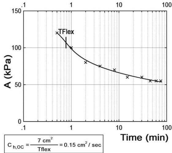
Fig. 7. DMT5 dissipation test at depth of 3 m [9]
