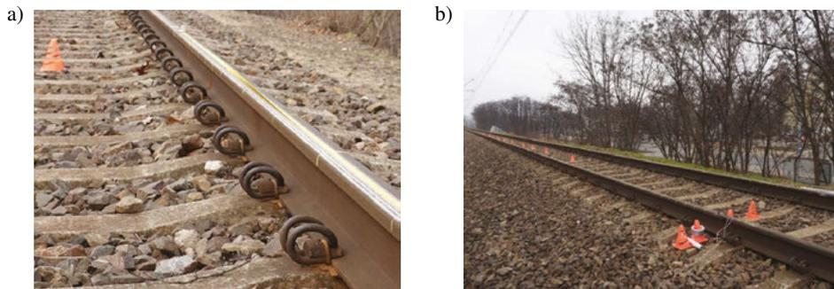
Fig. 3. Test field with marked sections selected for TDR tests: a) location of impulse excitation points, marked with yellow chalk; b) field ready for tests
