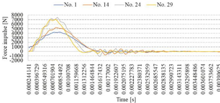
Fig. 10. Force impulse in the time domain registered by impact force sensors – horizontal excitations in points 1, 14, 24 and 29
