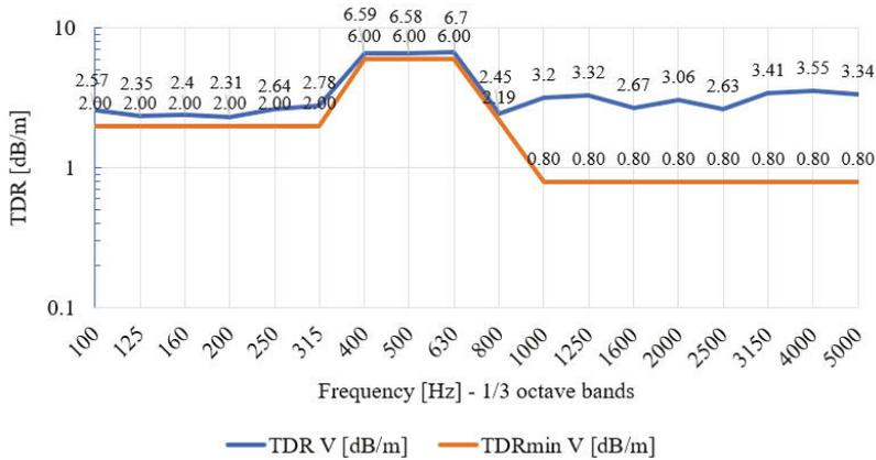
Fig. 14. Track decay rate (TDR) in vertical (V) plane – measurements series no. 2, rail no. 1 (N)
