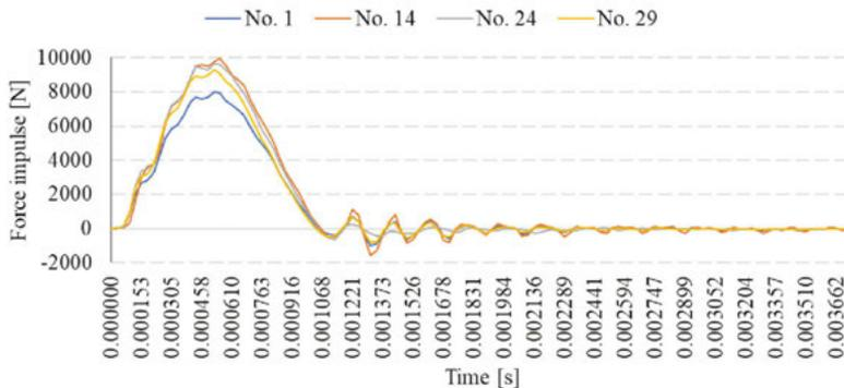
Fig. 6. Force impulse in the time domain registered by impact force sensors – vertical excitations in points 1, 14, 24 and 29
