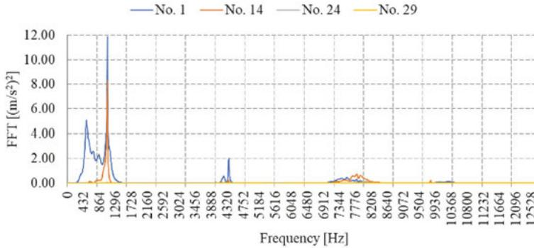
Fig. 9. FFT analysis of vibration accelerations – vertical excitations in points 1, 14, 24 and 29
