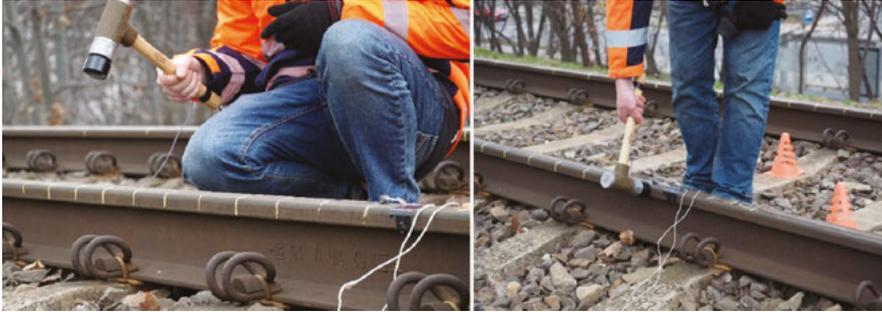
Fig. 5. Impulse excitation in the TDR test (left side: vertical, right side: horizontal)
