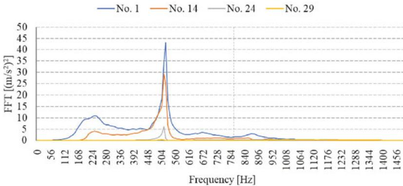
Fig. 13. FFT analysis of vibration accelerations – horizontal excitations in points 1, 14, 24 and 29
