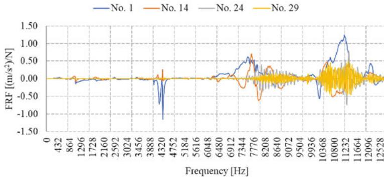
Fig. 8. Frequency response function (FRF) – vertical excitations in points 1, 14, 24 and 29
