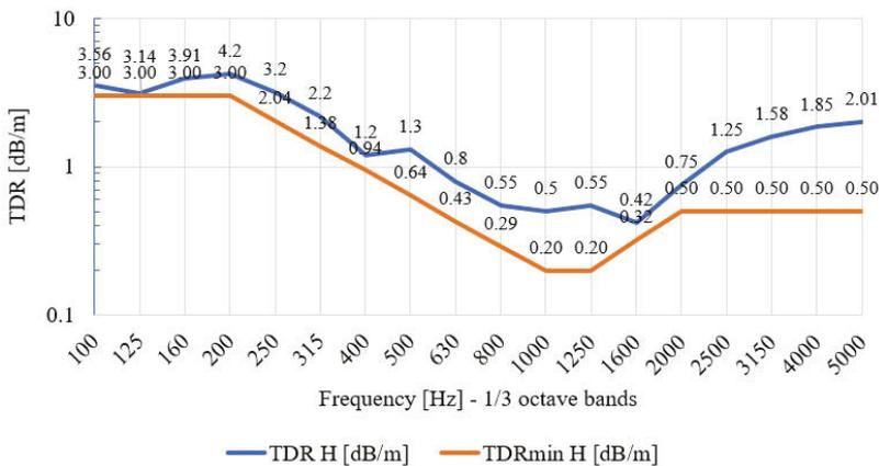
Fig. 15. Track decay rate (TDR) in horizontal (H) plane – measurements series no. 3, rail no. 1 (N)
