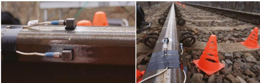
Fig. 4. Sensors installed on the rail during the TDR tests
