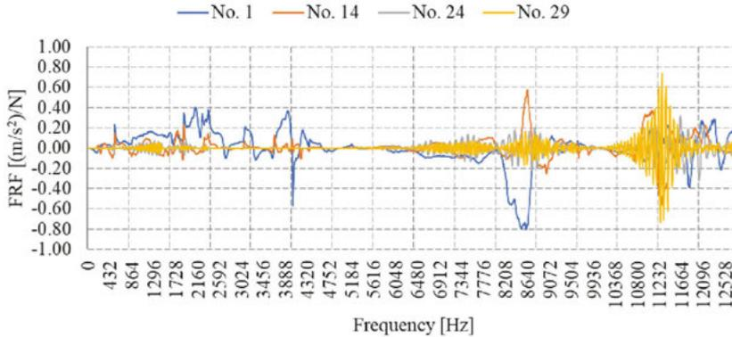
Fig. 12. Frequency response function (FRF) – horizontal excitations in points 1, 14, 24 and 29
