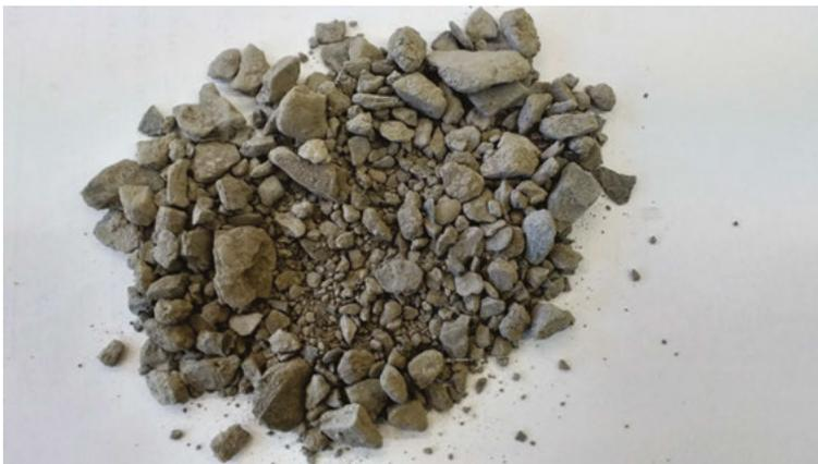
Fig. 1. Unburnt coal mining slate
