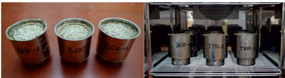
Fig. 3. Exemplary vessels with samples sealed (left); chamber providing constant conditions (right)
