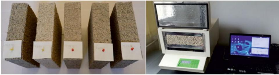
Fig. 2. Samples for thermal conductivity tests (left); FOX 314 plate apparatus (right)
