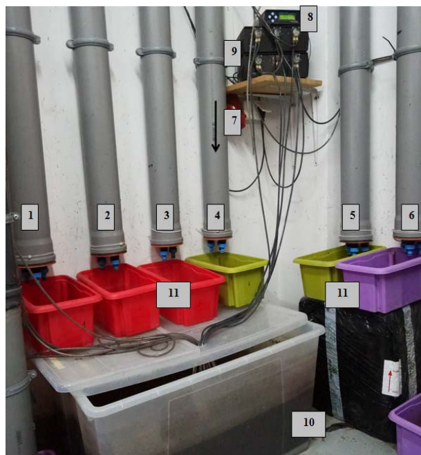
Photo 1. The column model; 1 = column with polyurethane foam, 2 = column with 60 cm sand, 3 = column with polyurethane foam, 4 = column with PET flakes, 5 = column with rubber tires, 6 = column with 30 cm sand, 7 = direction of sewage flow, 8 = time controller, 9 = peristaltic pumps, 10 = pretreated sewage in the septic tank, 11 = treated sewage (phot. inicjał imienia nazwisko autora fotografii)
