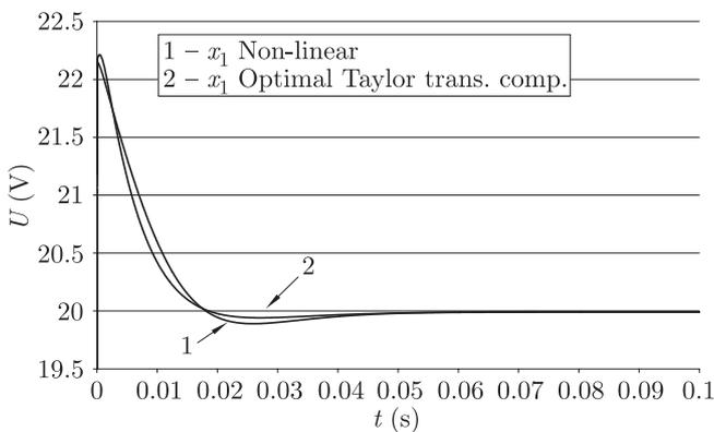
Fig. 10. The diagram of state variable  $x_1$  – comparison between solution of non-linear Eq. (8) and solution of optimal Eq. (22) based on Taylor's series expansion around the equilibrium point with the transient components
