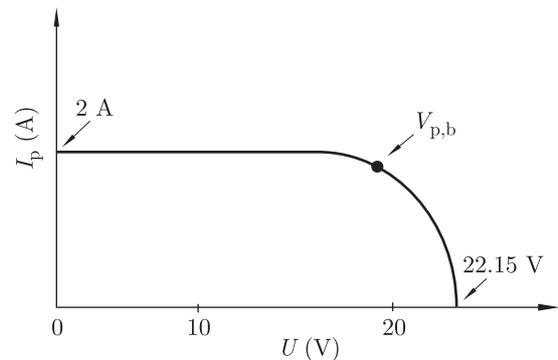
Fig. 2. Non-linear characteristic of solar generator.  $V_{p,0} = 22,15$  V is the generator voltage prior to switching on switch  $W$ .  $V_{p,b}$  is the equilibrium point of the system (steady state)
