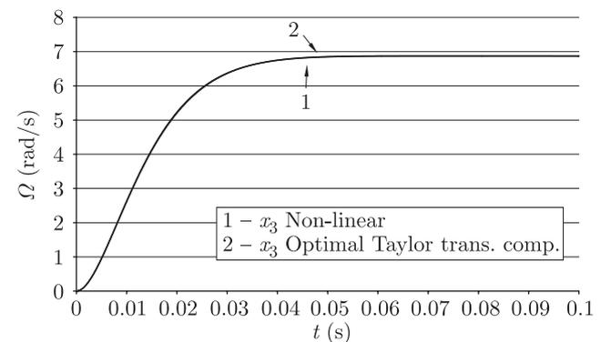
Fig. 14. The diagram of state variable  $x_3$  – comparison between solution of non-linear Eq. (8) and solution of optimal Eq. (22) based on Taylor's series expansion around the equilibrium point with the transient components
