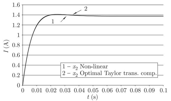
Fig. 12. The diagram of state variable  $x_2$  – comparison between solution of non-linear Eq. (8) and solution of optimal Eq. (22) based on Taylor's series expansion around the equilibrium point with the transient components
