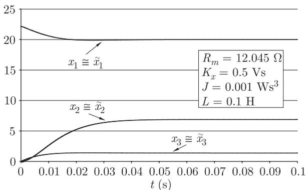
Fig. 16. The diagram presenting solution of linear equation with rated parameters and solution of linear equation with  $R_{m.1} = 3 \Omega$
