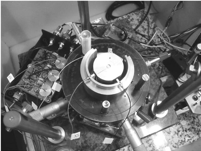
Fig. 4. Scanning Probe Microscopy scanning head with integrated 3 interferometers for measurements of piezoactuator deflection in XYZ directions
