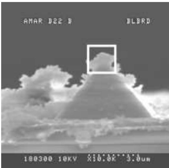
Fig. 8. Characterization of tip shape using  $\text{SiO}_2$  nanolines: 3D view of the topography structure a), zoom image of the single nanoline b), crosssection of the tip profile c), SEM image of the tested microprobe d)
