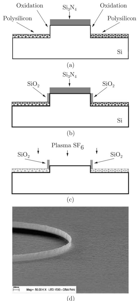
Fig. 7. Fabrication process of the calibration structure for the SPM tip characterization: oxidation of the sidewalls of the Si steps (a), oxidized Si steps before plasma etching of the Si<sub>3</sub>N<sub>4</sub> layer (b), plasma etching of the Si<sub>3</sub>N<sub>4</sub> layer and Si step (c), SEM image of the final device (d)
