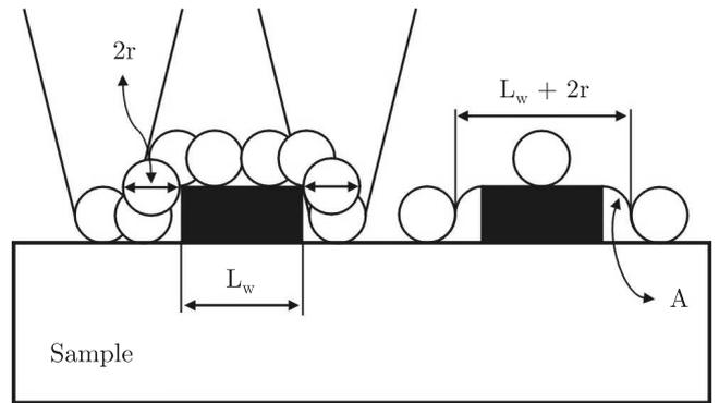
Fig. 6. Measurement of linewidth with the scanning probe microscope
