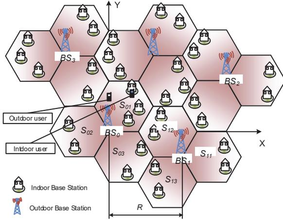
Fig. 1. 5G system model with OBSs and IBSs.
