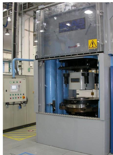
Fig. 3. Photograph of industrial hydraulic stamping machine for forming with the use of liquid
