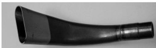
Fig. 1. A pressed element made of nickel superalloy by stamping and joining
