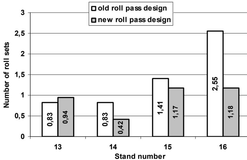
Fig. 6. Number of roll sets during three-strand rolling process of 16 mm ribbed bar about 90 000 Mg
