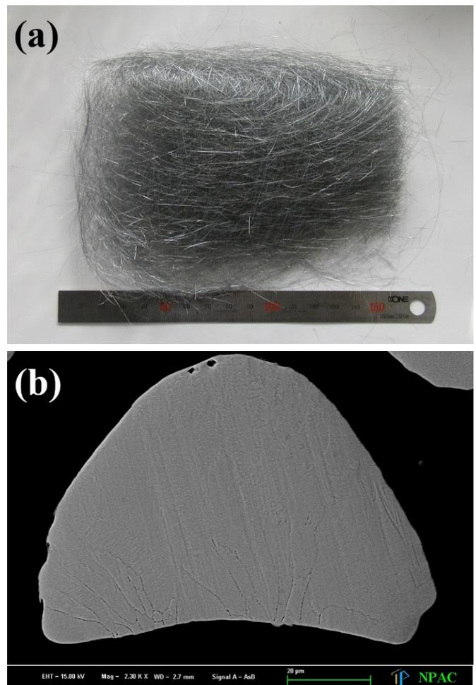
Fig. 1. (a) Photograph and (b) SEM micrograph of etched cross-section of as-solidified 77Ti-18Nb-5Mo fibers
