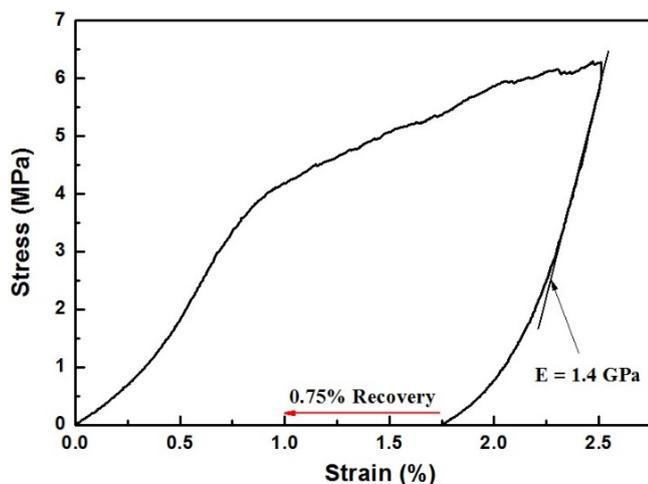
Fig. 5. Compressive strain-stress curve of porous 77Ti-18Nb-5Mo scaffolds
