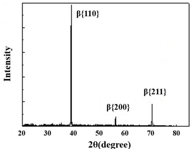
Fig. 4. XRD pattern of porous 77Ti-18Nb-5Mo scaffolds
