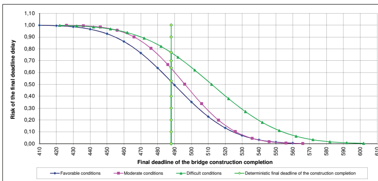
Fig. 1. Risk charts of the final deadline delay of bridge construction completion
