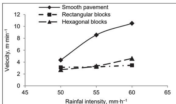
Fig. 3. Runoff velocity at slope of 15%; source: own study
