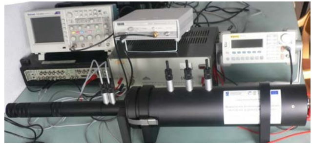
Fig. 4. Experimental setup for measurement of acoustic absorption coefficient of materials.
