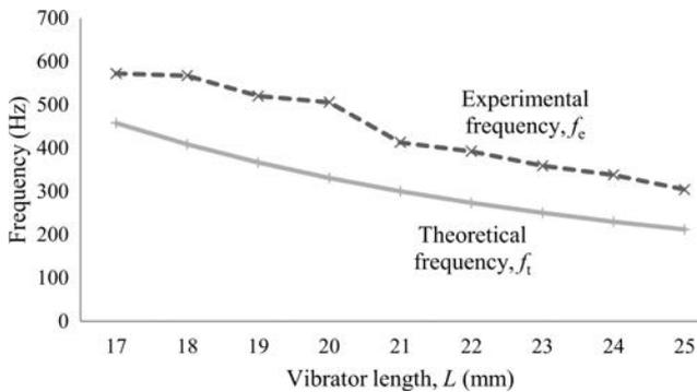
Fig. 6. Comparison between the theoretical SDOF using Eq. (7) and experimental values of the fundamental frequency of the aluminum vibrator of different lengths.
