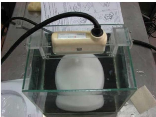
Fig. 4. US measurement methodology – a view of the tank.
