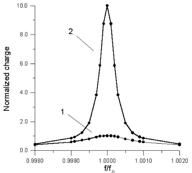
Fig. 5. Sharpening of the resonant curve of the OHC's electromechanical resonator due to the parametric amplification. Curve 1 – passive vibrations, curve 2 – active vibrations.  $f_0$  is a resonant frequency.
