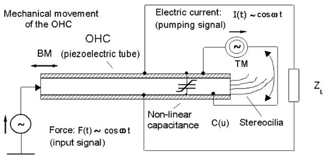
Fig. 1. Hypothetical simplified electro-mechanical diagram of a single OHC operating as a parametric amplifier.  $F(t)$  – represents the input acoustic signal,  $Z_L$  represents the electrical load impedance,  $C(u)$  – is a nonlinear capacitance.
