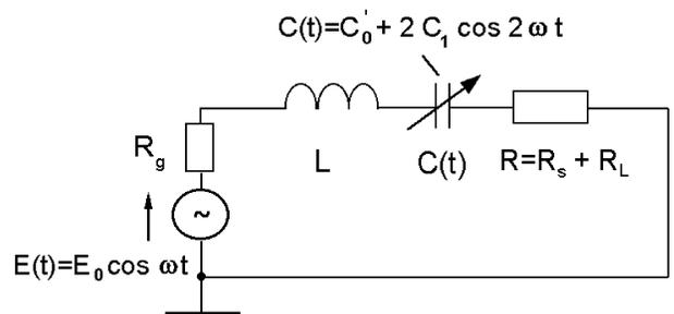
Fig. 3. Linearized (lumped-element) Thevenin electrical equivalent circuit of an individual OHC operating as an electromechanical resonator.
