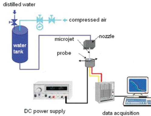
Figure 1. Schematic diagram of test section.
