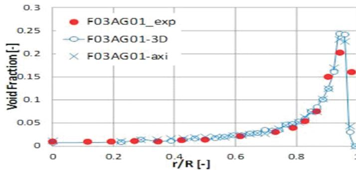
Figure 11. Void fraction profile for run F03G01,  $j_f = 2$  m/s,  $j_g = 0.209$  m/s. The solid circles denote the experimental results, the open circles are the calculated ones with the 3D Eulerian code and the crosses (x) denote the calculated with the 2D Eulerian solver. Both calculation were performed with  $C_{Ib} = C_{Ib0}$ .
