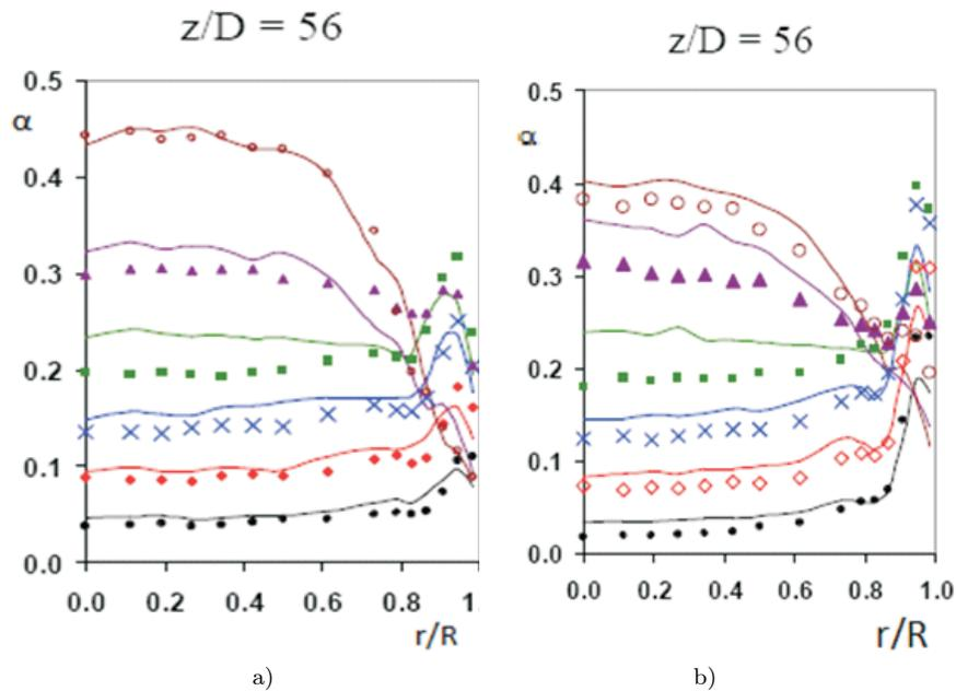
Figure 9. Test results for different gas superficial velocities at  $z/D = 56$ : a) for runs D01 and B01; b) for runs D02 and B02.
