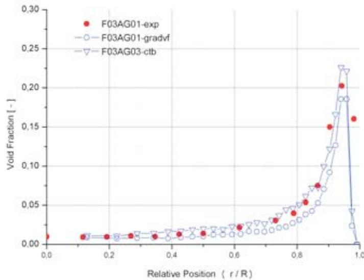
Figure 10. Void fraction profile for run F03G01,  $j_f = 2$  m/s,  $j_g = 0.209$  m/s. The solid circles denote the experimental results, while the open circles are the calculated ones with  $C_{Ib} = C_{Ib1} + C_{Ib2} \nabla \alpha$ , and the triangles the calculated with  $C_{Ib} = C_{Ib0}$ .
