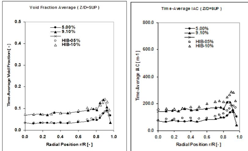
Figure 7. Comparison of experiments performed by Hibiki, Ishi and Xiao for the void fraction and the interfacial area concentration [25], with the experimental results of Chiva *et al.* [26], for the conditions of experiments F01G01 and F01G02, displayed in Tab. 1.
