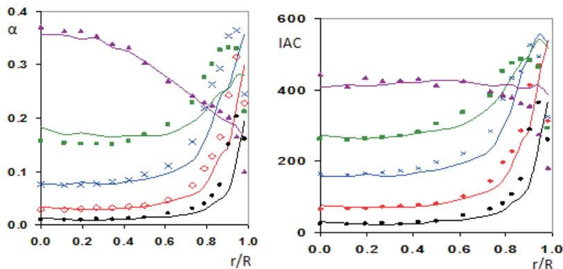
Figure 8. Void fraction versus  $r/R$  and IAC versus  $r/R$  for case FO3 with  $j_f = 2$  m/s, at the upper port  $z/D = 56$ . Solid symbol correspond to F0A probe configuration, and without symbol (continuous line) to F0X probe. Black ( $\bullet$ ) G01, Red ( $\diamond$ ) G02, (X) G03, Green ( $\blacksquare$ ) G04, Violet ( $\blacktriangle$ ) G05.
