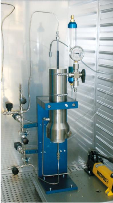
Fig. 3. Hassler type core holder
