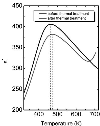
Fig. 3. Real part of permittivity as a function of temperature measured on heating at frequency of measuring field 100 kHz for sample of  $\text{BaBi}_2\text{Nb}_2\text{O}_9$  ceramics before and after thermal treatment at 1173K in the ultra high vacuum
