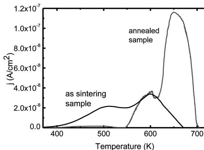
Fig. 5. Thermally stimulated depolarization currents vs. temperature for BBN ceramics before and after thermal treatment at 1173K in the ultra high vacuum
