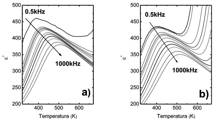
Fig. 4. Real part of permittivity as a function of temperature and frequency of measuring field 100kHz obtained on heating for  $\text{BaBi}_2\text{Nb}_2\text{O}_9$  ceramics a) before and b) after thermal at 1173K in the ultra high vacuum treatment
