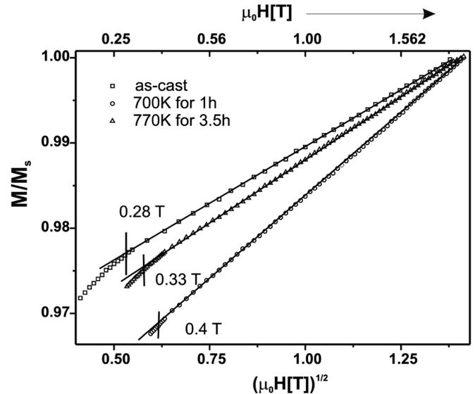
Fig. 5. Reduced magnetization  $M/M_S$  of the  $Fe_{61}Co_{10}Y_8Zr_1B_{20}$  alloy, in the as-cast state and after heat treatment as a function of  $(\mu_0 H)^{1/2}$
