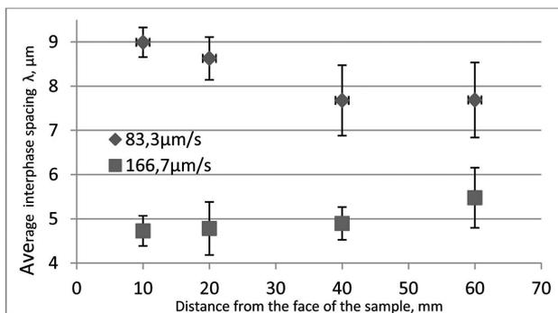
Fig. 7. The dependence of average interphase spacing  $\lambda$  on growth rates  $v$  at a constant  $G = 33,5$  K/mm
