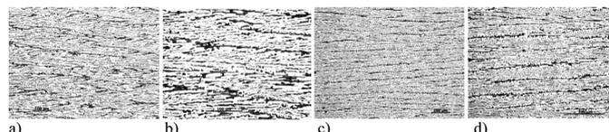
Fig. 4. Microstructure of directionally solidified Fe-Fe<sub>3</sub>C eutectic alloy on the longitudinal section of each samples,  $G = 33,5 \text{ K/mm}$ , a,b)  $v = 83,3 \mu\text{m/s}$ , c,d)  $v = 166,7 \mu\text{m/s}$
