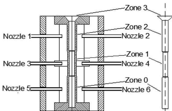
Fig. 1. Section of mold and casting, zones and nozzles
