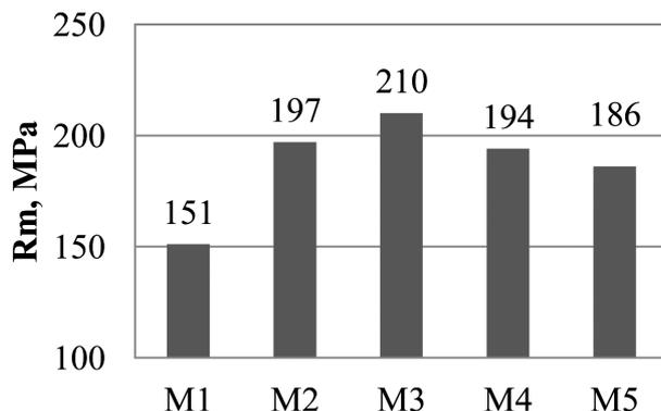
Fig. 6. Influence of cooling method on the tensile strength  $R_m$  of casts
