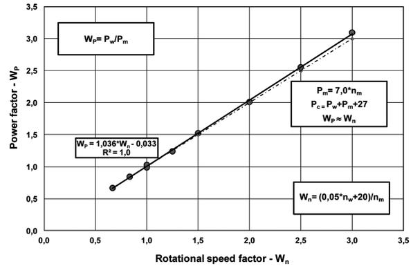
Fig. 6. Power uptake by the rotor and pan drives  $W_p$  versus the drive rpm factor  $W_n$  (tests include the idle run of the mixer- dimensionless coordinates)
