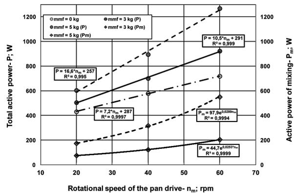
Fig. 8. Active power uptake by the mixer drives under the steady-state operational conditions in the function of a variable pan drive’s rpm speed  $n_m$  during the duty cycle: pan load: 3 and 5 kg of sand, rotor’s rotational speed:  $n_w = 400$  rpm.
