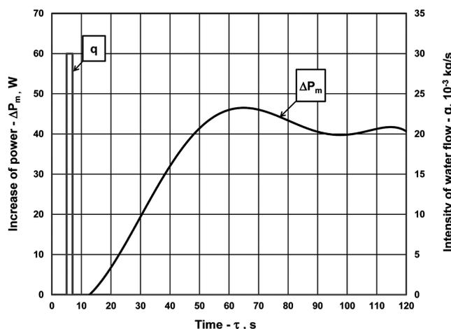
Fig. 9. Time run of increase of active power connected with moulding sand mixing and simultaneous water dosing; load of the pan: 3 kg of moulding sand, change of moisture value  $\Delta W = 2\%$ . ( $n_w = 600$  rpm,  $n_m = 40$  rpm, run of power signal – trendline for mean values, intensity of water flow – approximated by rectangular pulse)
