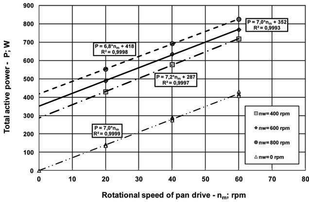
Fig. 4. Active power  $P$  intake by the mixer drives under steady –state conditions in the function of the variable rpm of the pan drive  $n_m$
