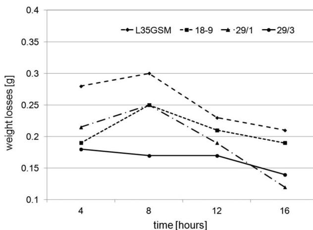
Fig. 6. Changes of weight losses of investigated cast steels during the wear test
